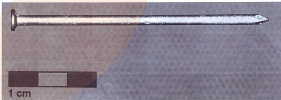
tested nail 3,40 x 90 mm smooth HDG
