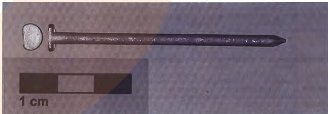
tested nail 2,90 x 65 mm smooth HDG
