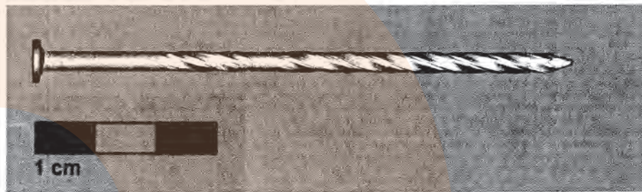
tested nail 3,10 x 90 mm spiral HDG
