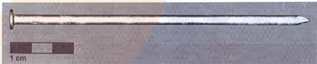
tested nail 4,60 x 145 mm smooth HDG
