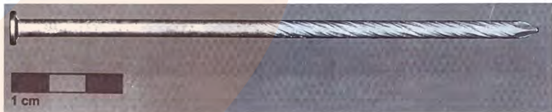
tested nail 4,60 x 145 mm spiral HDG
