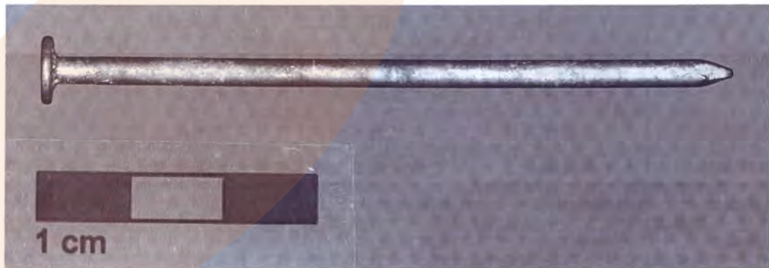
tested nail 2,90 x 75 mm smooth HDG
